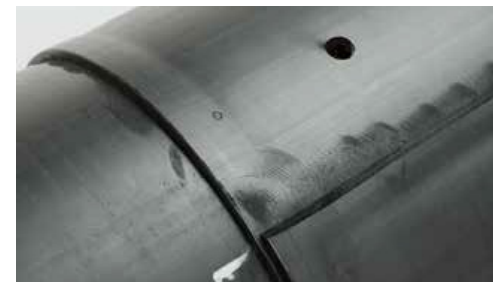
Visual inspection is possible. A filled hole indicates correct fusion and welding.
