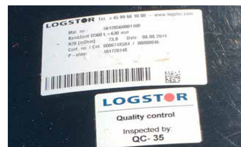
This provides reliable data for correct automatic configuration of the welding process.
